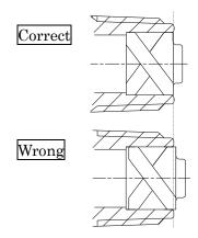
When correctly set, the whirler is positioned deeper than the rear end of the nozzle body as shown in the figure.
