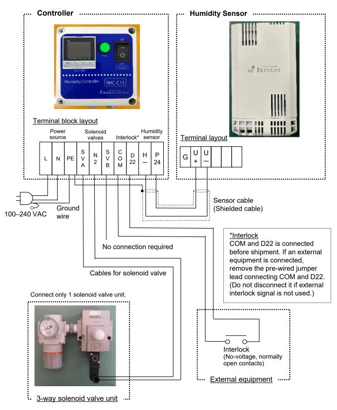
Note: Use a solenoid valve with the same voltage specification as the input voltage.
