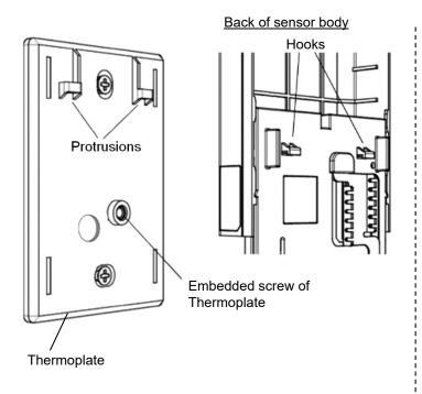
It is easier if you hold the sides of the sensor body with both hands, press down slightly, and slide it downward.
