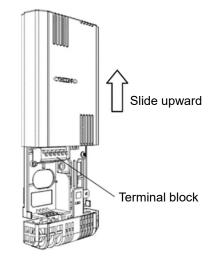
iii. Hook the back hooks of the humidity sensor onto the protrusions of the thermoplate mounted on the wall.
