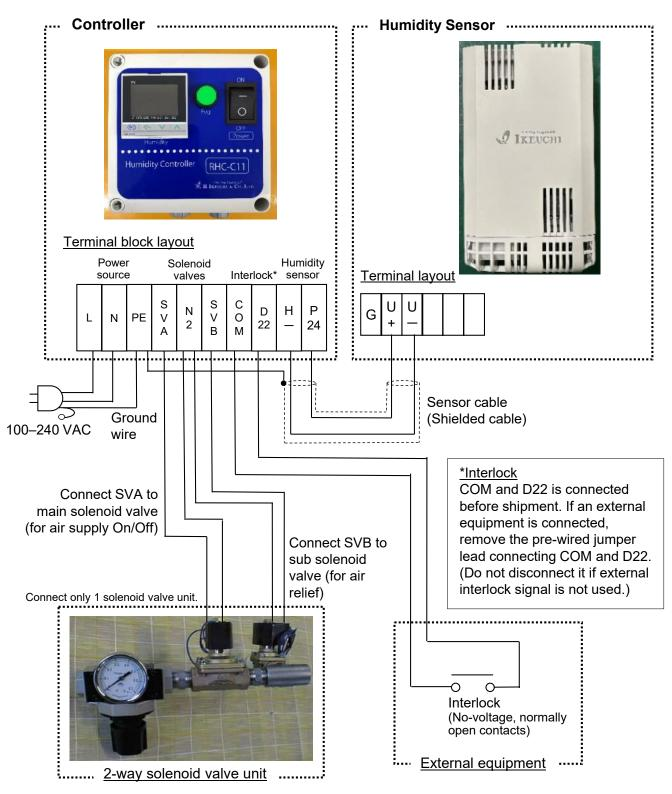
Note: Use a solenoid valve with the same voltage specification as the input voltage.
