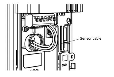
ii. Connect the sensor cable to the second and third terminal blocks from the left. While pressing down on the protrusion in the upper part of the terminal block, insert the stripped end of the cable into the insertion slot and then release the protrusion.
