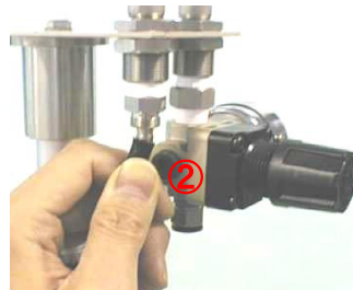
Slip the fitting cap on the black tube and insert the tube fully into the fitting.
