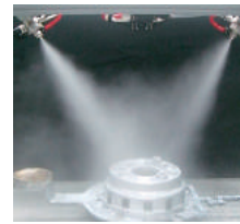
Die-cast and cast product cooling system
