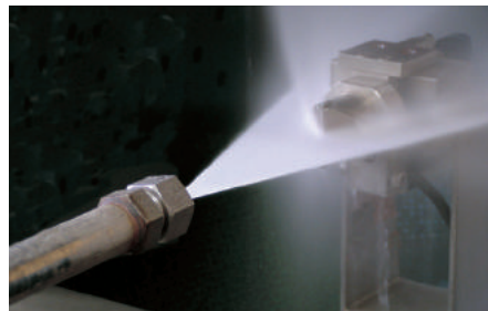
Spray impact measurement
