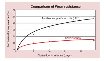
Shown on the right is the comparison of test results between the UVVP series flat spray nozzle and a UPE nozzle made by another manufacturer.
