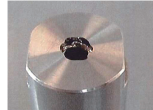
Orifice worn out by slurry
